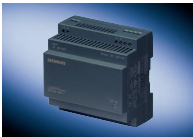
LOGO!Power supplies are primary switched-mode power supplies that are optimized to the LOGO! logic modules in terms of functionality and design. With the wide input range of 85 V to 264 V AC, radio interference level B and assembly option in built-in miniature distribution boards, they can be used universally in a diverse range of applications in the low-end performance range.
